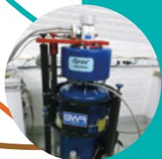
iOSG supraconducting gravimeter
